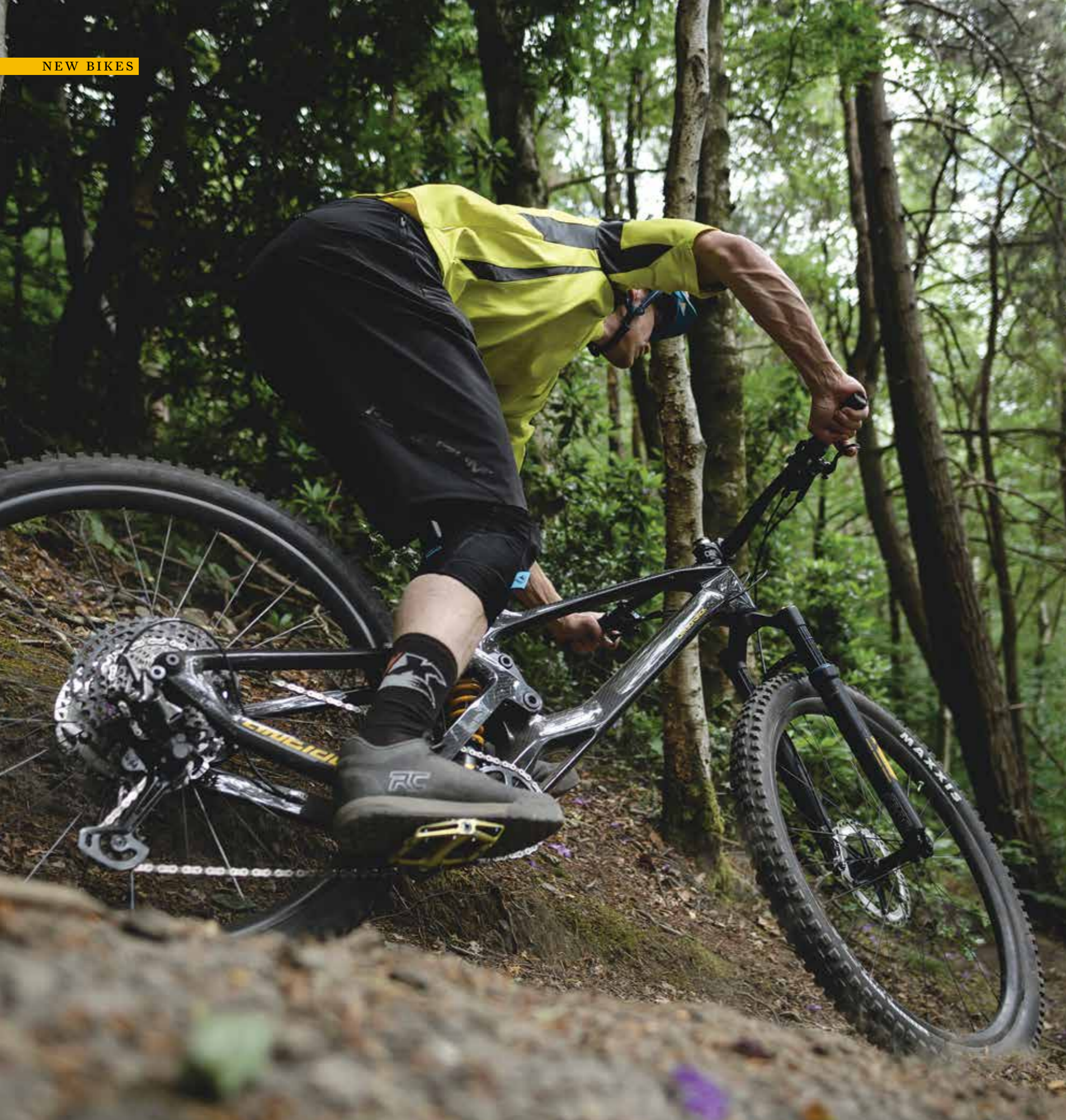
150mm-travel Öhlins TTX coil shock perfectly tracks the trail
